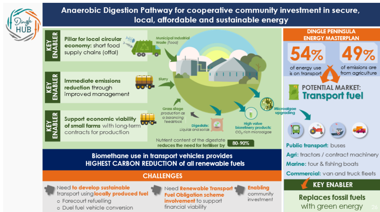
Fig 2. Anaerobic Digestion Pathway for cooperative community investment in secure, local, affordable and sustainable energy
