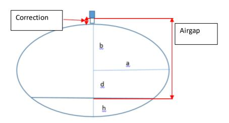
Air Gap is the distance between the sensor and the top of the milk.
